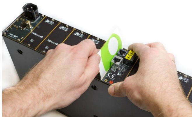
Figure 16: Inserting a new back plane.
