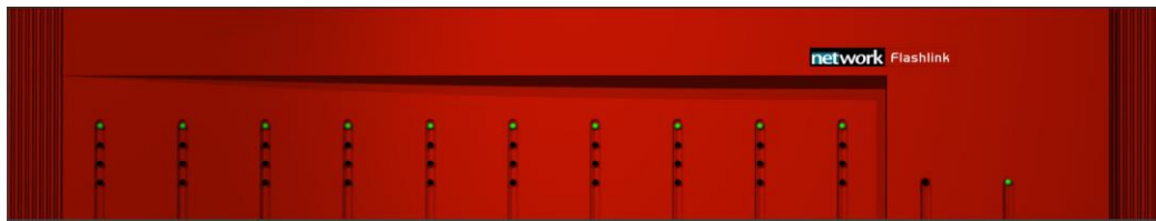
Figure 1: LEDs in front of the Flashlink sub-rack.
