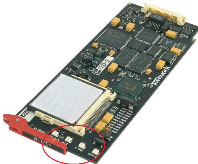
Figure 12.4 LEDs on Multicon hardware revision 2
