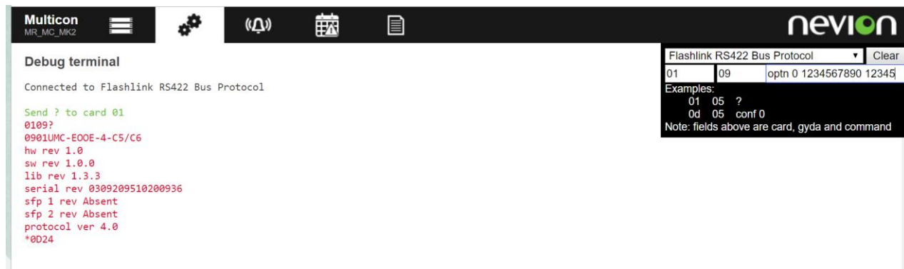
Figure 37: The debug terminal, ready to send the software key to the module
