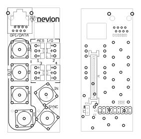
Figure 4: FRS-HD-XMUX4-C1 backplane left: connection side right: component side
