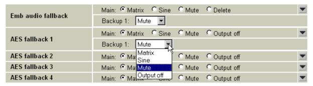
Figure 16: Multicon GYDA view of the audio fallback options
