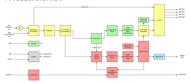
Figure 1: Simplified block diagram of the FRS-HD-XMUX4 card
