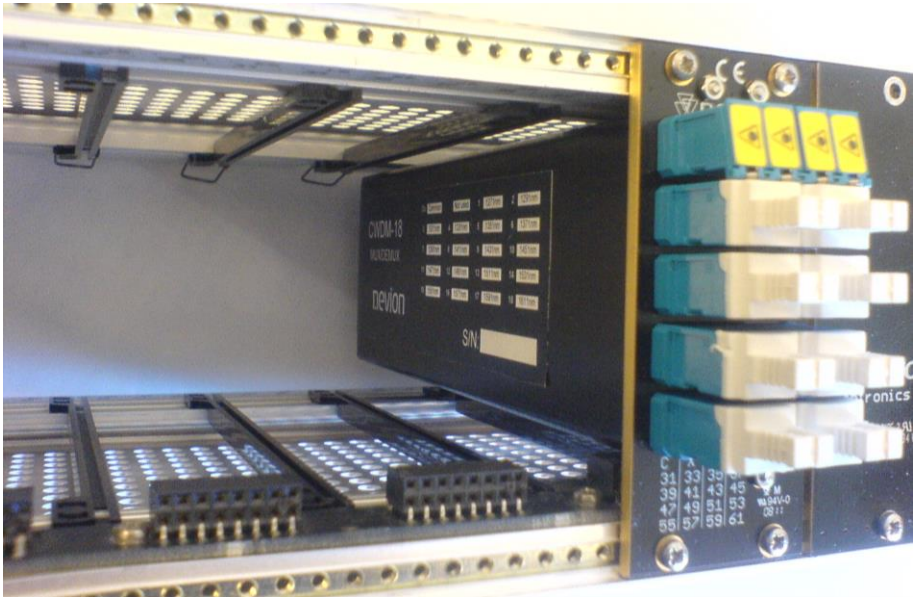
Figure 8 Module mounted in frame
