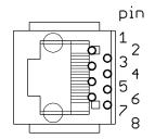
Figure 7: Pin layout 8P8C Modular jack
