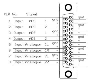
Figure 6: DB-25 audio connector wiring
