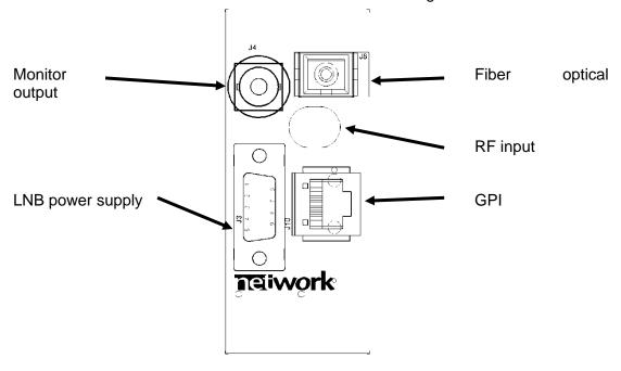
Figure 3: Connector module for L-band.
