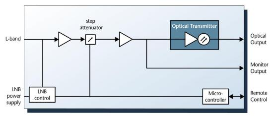
Figure 1: LB-EO L-band electrical to optical converter.
