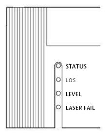
Figure 5: Front panel indicators for the LB-EO.
